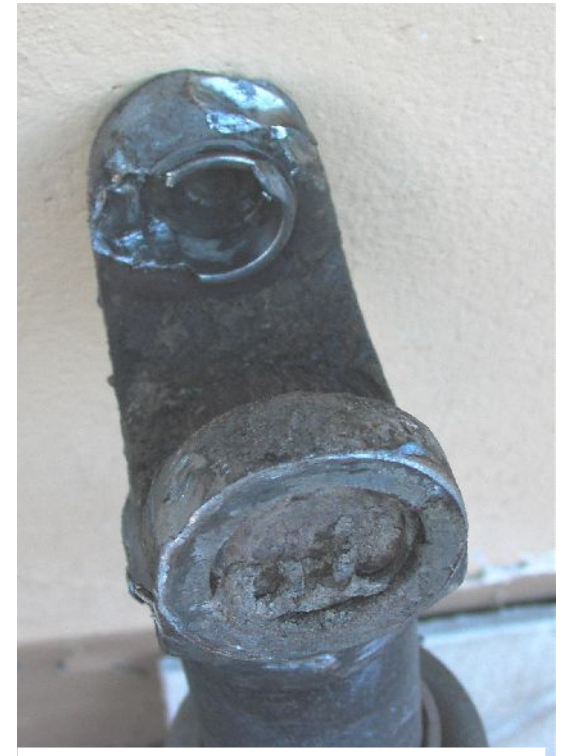
The broken end of the drive shaft from the Land Rover.
